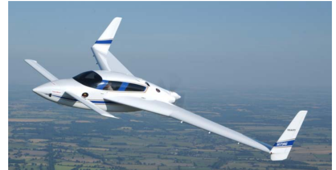
Velocity - advanced home-built from epoxy resin and carbon fibre
