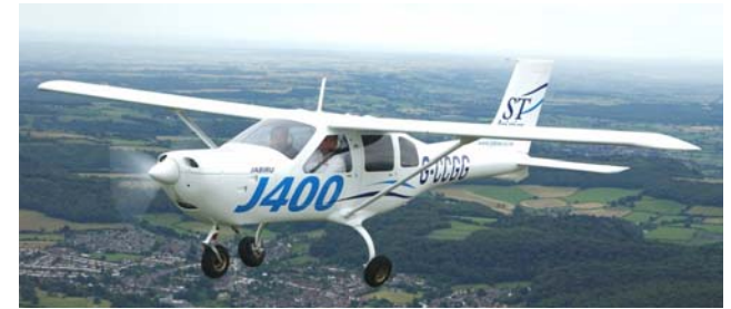
Jabiru J400 - Australian designed 4-seater composite kit-plane
