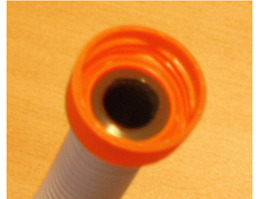
Pipe insert fitted in position in the drilled bottle cap
